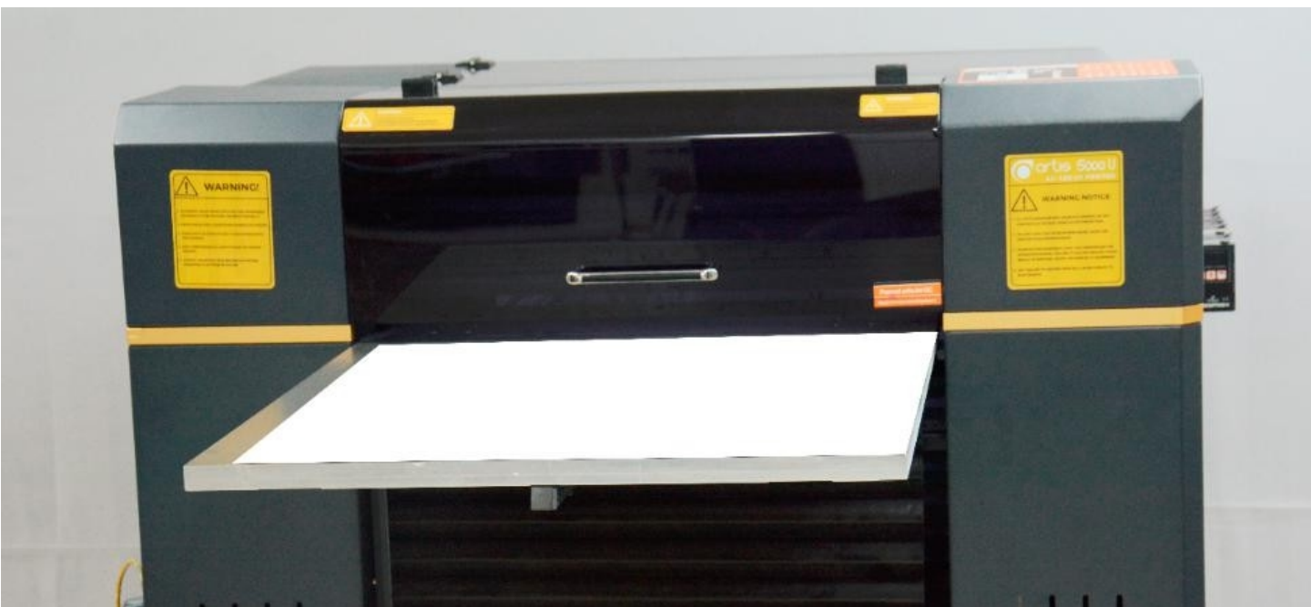
Fig.25 – Put the E-fixture mat onto the table and spread it till even on the surface
