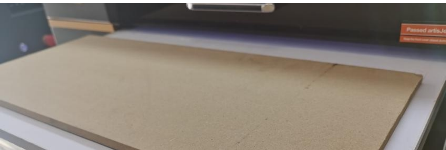
Fig.39 – Place product on the working table; it must be in front of the height sensors
