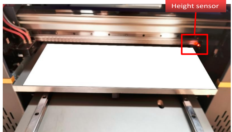
Fig.26 – automatic height adjustment with height sensor
