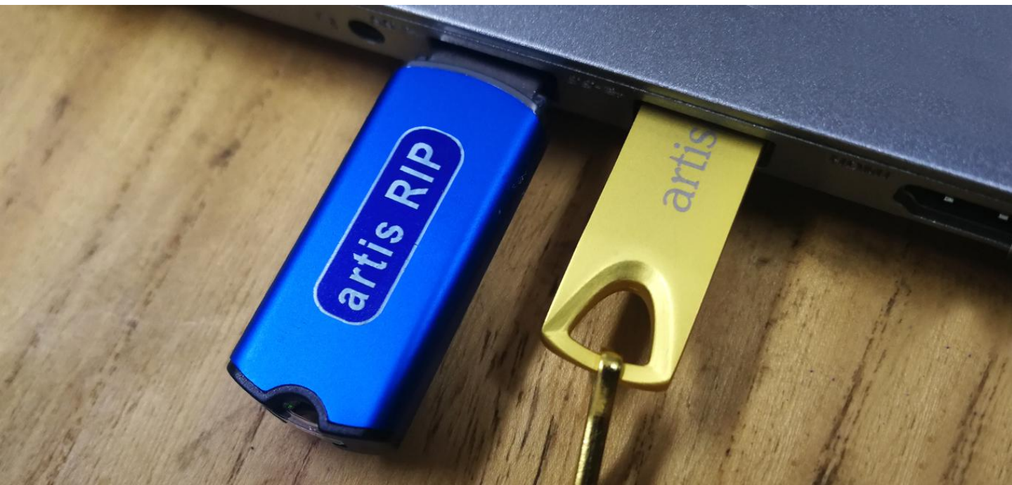
Fig.14 – Insert the USB drive (artis 3000U pro) & the Design Software dongle (artisRIP V9.0)
