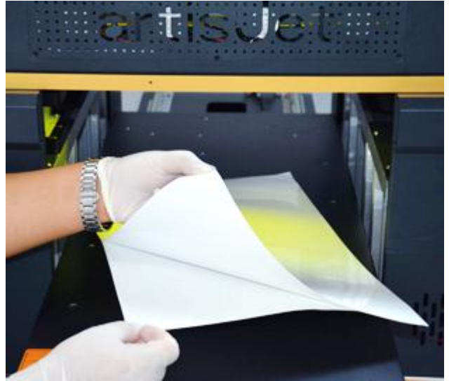
Fig.24 – Take one piece of E-fixture matt and peel off the film one side only
