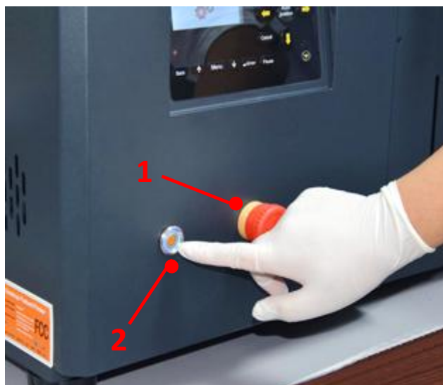
Fig.11 – Turn on the printer - 1. Unlock the emergency switch; 2. Press General power button
