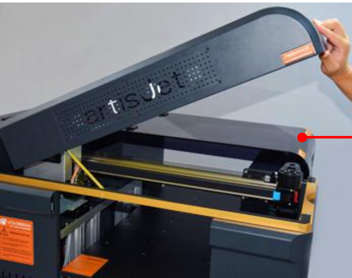
Fig.8 – Open the cover carefully and take out the E-fixture matt from the working table
