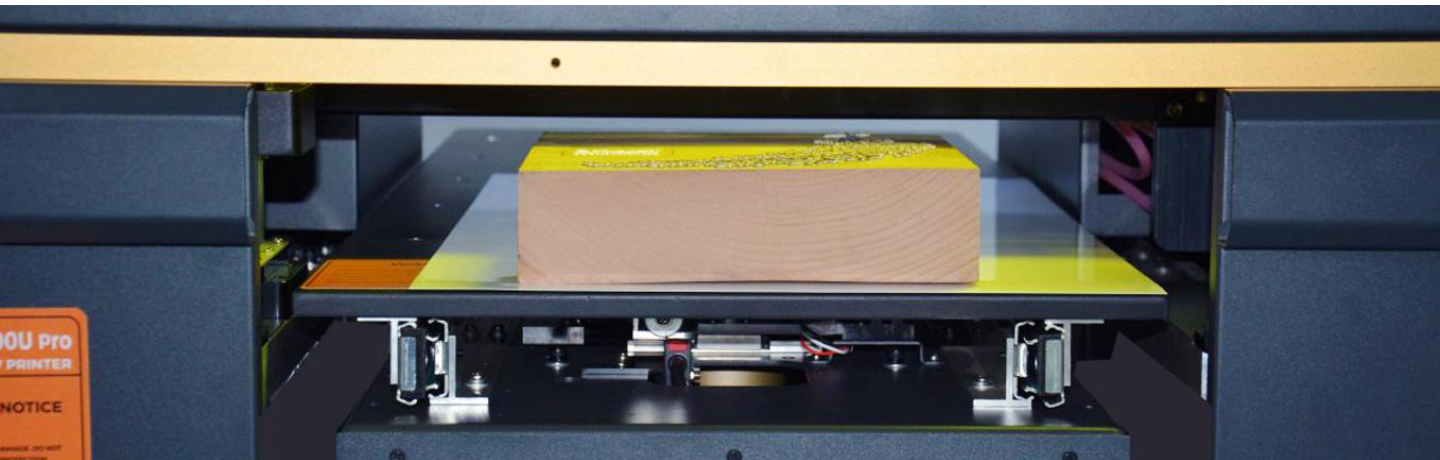
Fig.40 – Auto-detecting the sample and auto-adjusting the printing height
