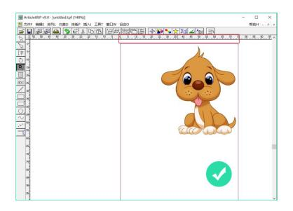
Unreasonable page size settings will increase the excessive movement of the carriage during printing, increasing more print time and the frequency of UV lamp lighting.
