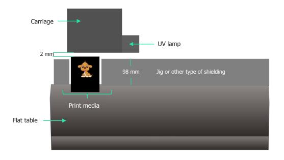
**b.** Set the width of page size with proper value and adjust the placement position of print media on the flat table to effectively avoid this kind of reflection.
