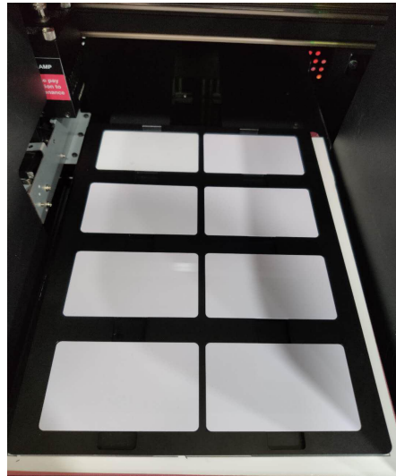
Card position on the template
