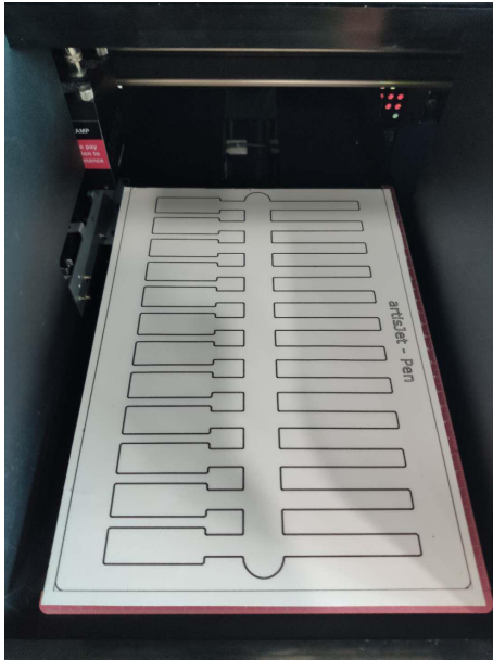
Pen template print position on the flat table
