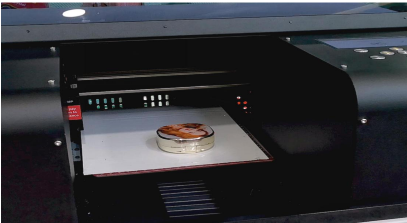
Fig.33 – Auto-detecting the sample and auto-adjusting the printing height
