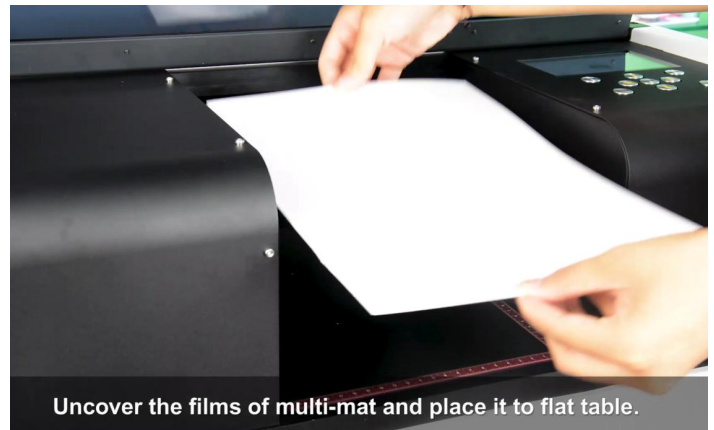
Fig.20 – Take one piece of E-fixture matt and peel off the film one side only
